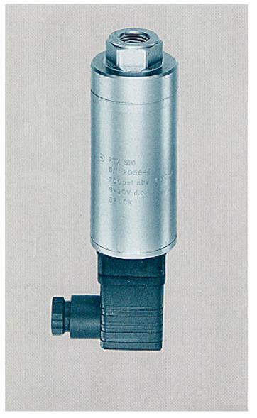
The PTX 500 series combines micro machined silicon diaphragms with fully welded stainless steel and Hastelloy pressure ports to provide a highly accurate, stable pressure transmitter with the materials and environmental protection required for industrial applications.
