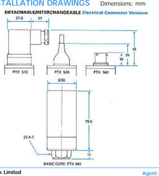
(1) Type number PTX 5X X = X Approvals (or omit) Commercial I Intrinsically safe **Temperature Effects** 0 -10° 10 -50°C 1 -20° to +80°C **Electrical Connection** Solder tags (IPS0) DIN 43550 plug/socket (IP65) Integral cable assembly (IP63) Submersible cable assembly (IP68 to 700mH,0g) Potatable conduit (IP65) M20 conduit (IP65) M12-C-26482 plug/socket 0 23
